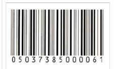
Incorrect adjustment for ink spread. The bars are out of specification (being too wide or too narrow)
