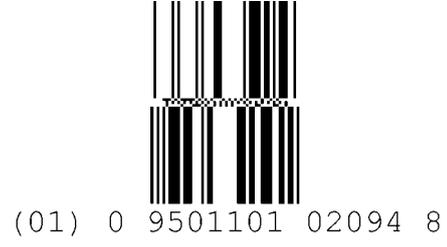
**GS1 DataBar Stacked Omnidirectional**
