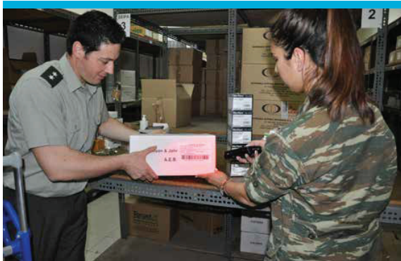
As products arrive, warehouse personnel scan each carton's GS1-128 barcode to capture product information in the warehouse management system.
