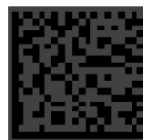
Figure 3.6.1.2-1 A symbol with very poor Symbol Contrast.
