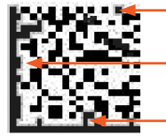
Figure 3.6.1.2-2 A Symbol with poor Modulation caused by irregular dark areas
