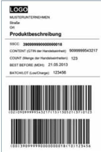
This pattern of a Logistics Label demanded by METRO contains a GS1-128 barcode encoded with the SSCC and GTIN of a singular type of product loaded on the pallet. The label shows 123 cartons of the product with the batch/lot number and best-before date.
